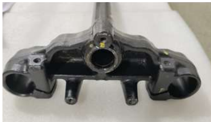
Failed Bracket shaft assembly
