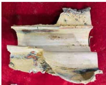
Failed Boiler Bank Tube
