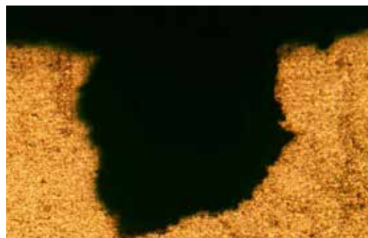
Microphotograph of Pitting corrosion
